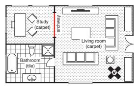
If there was damage to the flooring at the spot marked 'X' in the living room, we would only repair or replace the flooring within this functional area. In this scenario, we may need to introduce a floor trim between the study and living room as per the red line, since the damage is contained within the living room alone.
