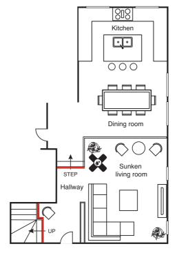
If there was damage to the flooring at the spot marked 'X' in the sunken living room, we would only repair or replace the flooring within this functional area up to the red line. In this scenario, we may need to introduce floor trims at the base of the steps along the red lines.
