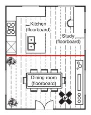
If there was damage to the flooring at the spot marked 'X' in the dining room, we would only repair or replace the flooring within this functional area up to the red line. In this scenario, we may need to introduce a floor trim along the red line
